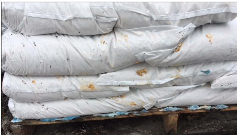
Figure 9. Messy and undesirable blue and yellow crystal creep from the YPS treated salt.
